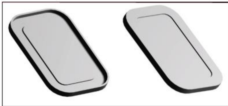
Figure 1: 3D Model of Food Container Lid
