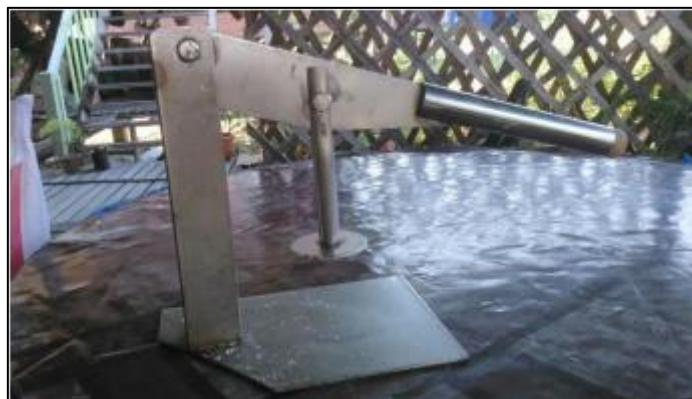
Figure 1: A Traditional Wet Sago Starch Compressor
