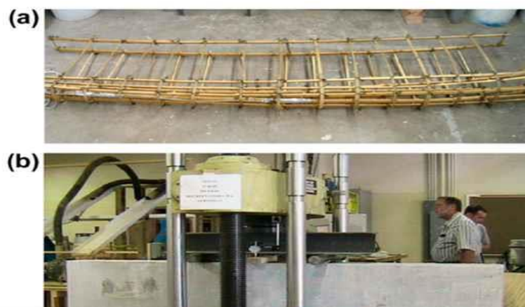
Figure 9. Concrete Beams Reinforced With Bamboo Rebars: (A) Finished Reinforcement, (B) The Setup
