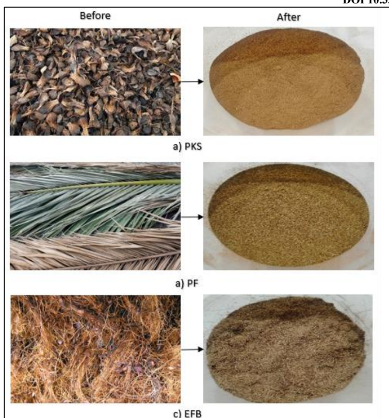
Figure 1: Palm Wastes Powder Prepared For Extraction; a) PKS, b) PF, c) EFB
