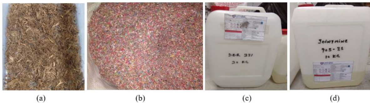
Figure 1: (a) PEFB Fibers (b) LDPE Plastic Waste (c) Epoxy Resin (DER-331) (d) Hardener (Jointment 905-3S)
