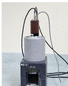
Figure 6: A Gamma-Ray Spectrometer Used for Radiation Characterization
