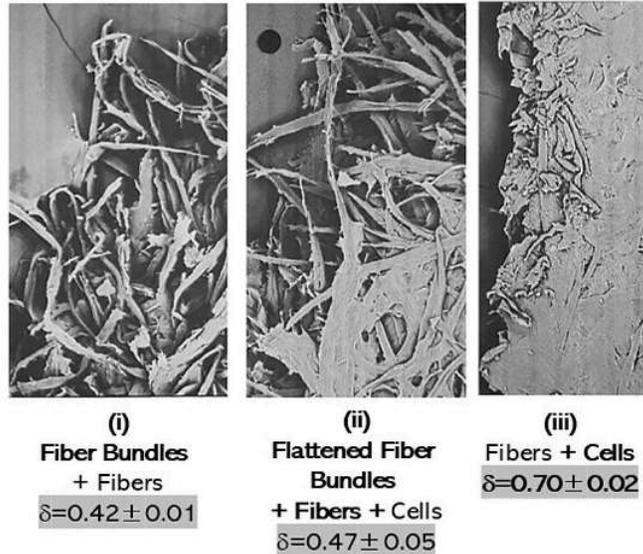
**Figure 4. Transitional Optical and Physical Properties with Images of the Torn 60 GSM Web Strip-Edges for  $\mu$ fibre (i),  $\mu$ fibre+TRX Mix (ii), and TRX (with Parent Fibre (iii)).**
