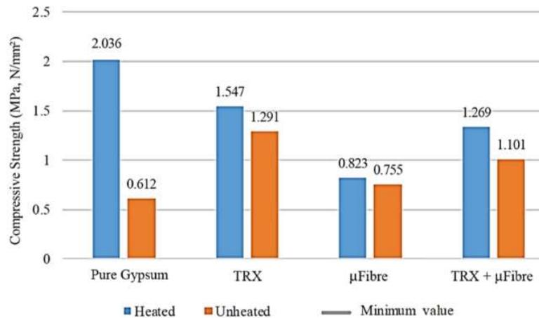
**Figure 3. Compressive Strength of the Modified Recycled Gypsum.**
