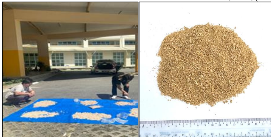
Figure 5: Drying process of Sago Fibre (left) and Sago Fibre after drying process (right)
