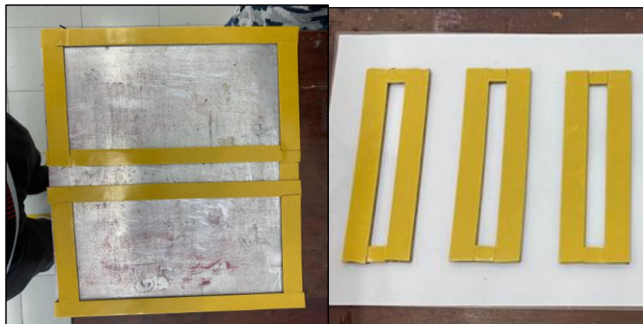
Figure 5: Tensile Test Sample Mould (left) and Flexural Test Sample Mould (right)
