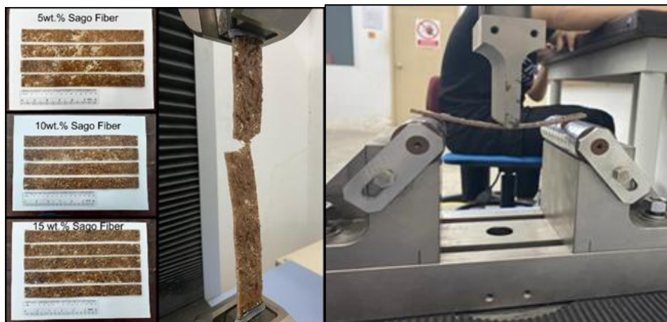
Figure 7: Tensile Test (left) and Flexural Test (right)
