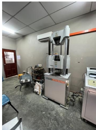
Figure 7: Compressive Strength Test
