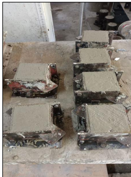
Figure 5: Casting of Concrete Cube Sample
