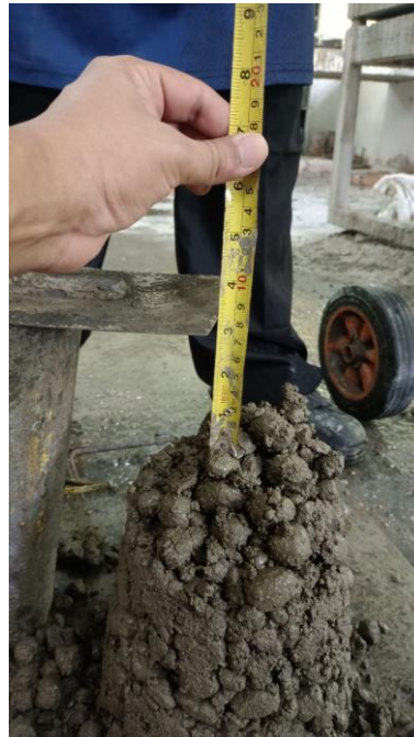
Figure 7: Slump Test on Fresh Concrete
