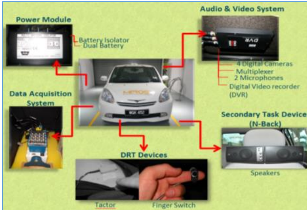
Figure 1: Instrumented Car Set-Up
