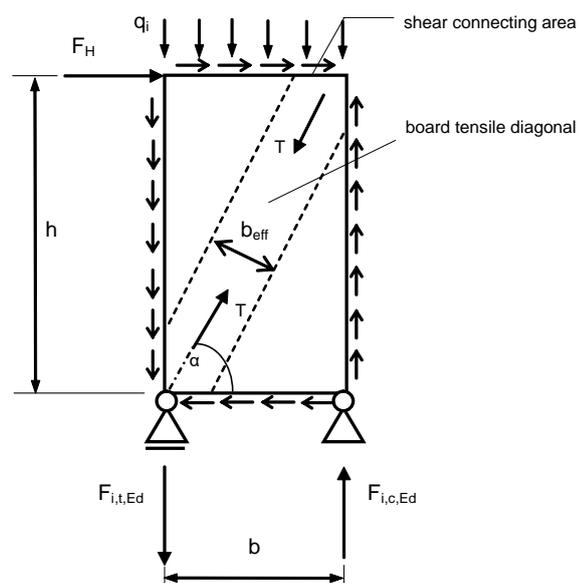
**Figure 7: Schematic Presentation of The Stress Transfer in Timber-Frame Wall Element Under A Horizontal Load ( $F_H$ )**
