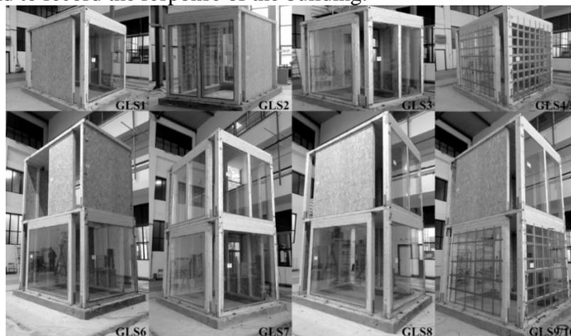
**Figure 12: Configuration of One-Storey and Two-Storey Test Models,** Source: Premrov et al. (2014)
