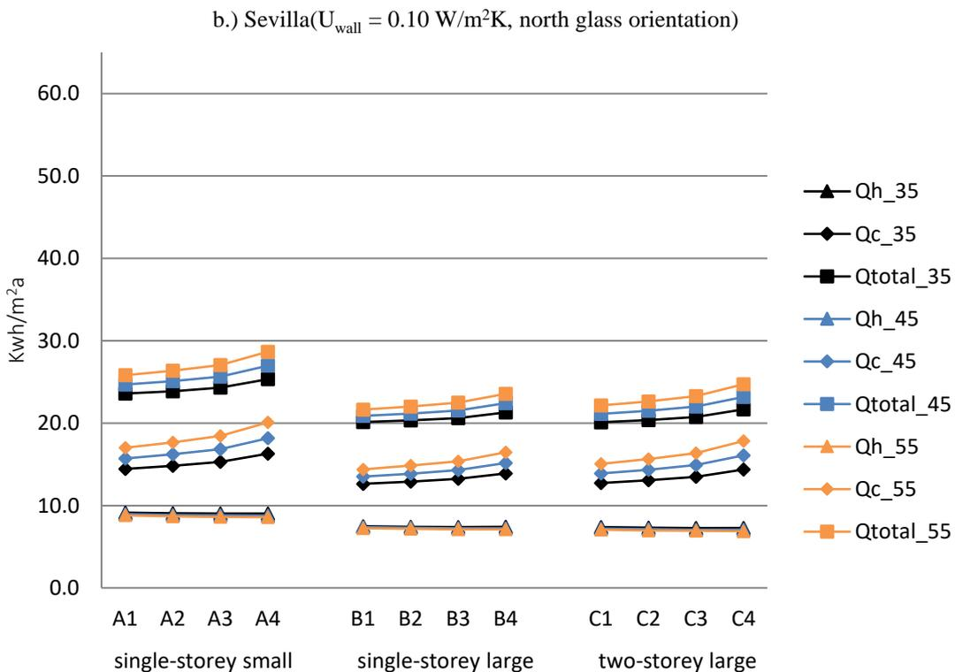
**Figure 6: Calculated Results For The Heating ( $Q_h$ ), Cooling ( $Q_c$ ) and Total Annual Energy Need ( $Q_{\text{total}}$ ) for Sevilla by South-oriented Glazing and Same Thermal Transmittance**
