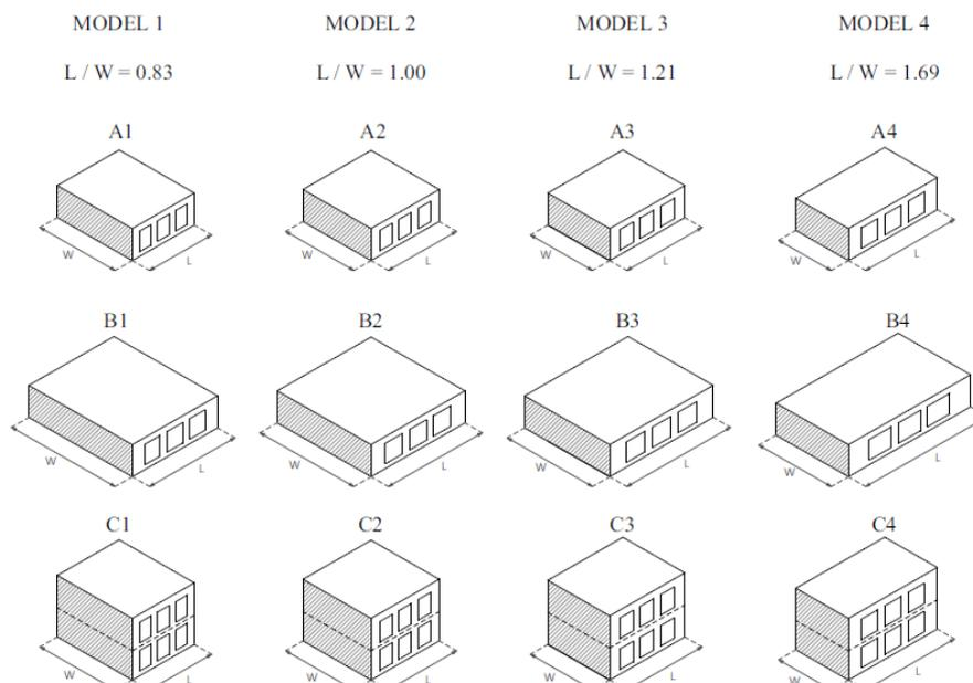
**Figure 5: Schematic Presentation of The Analysed Box-House Models**, Source: (Premrov et al., 2018)
