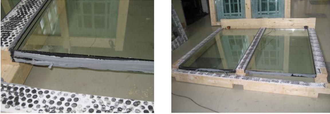
**Figure 9: Photo of The Collapsed Test Samples**
