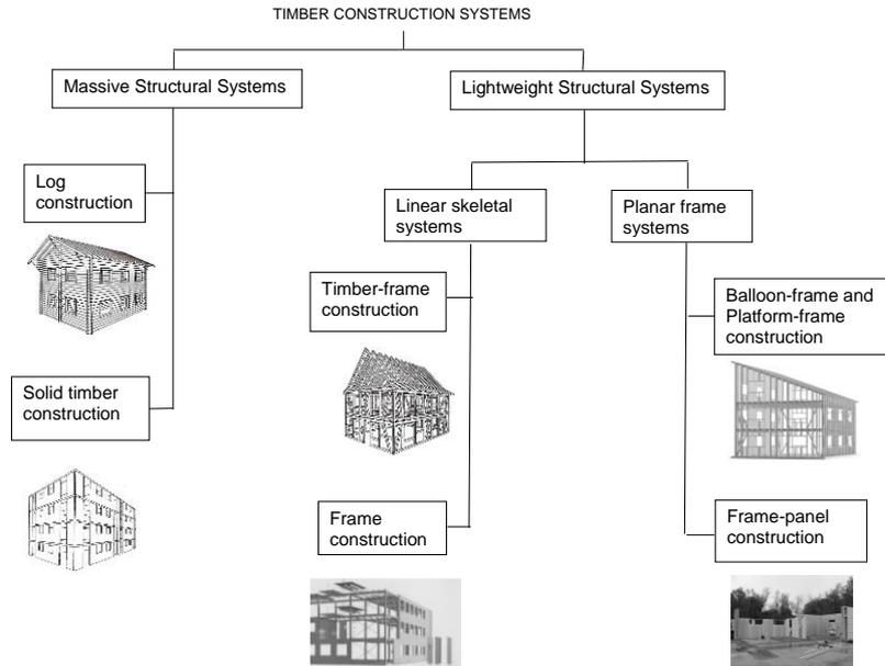
**Figure 3: Classification of Timber Structural Systems According to Their Load-Bearing Function,** Source: (Žegarac Leskovar and Premrov, 2013)
