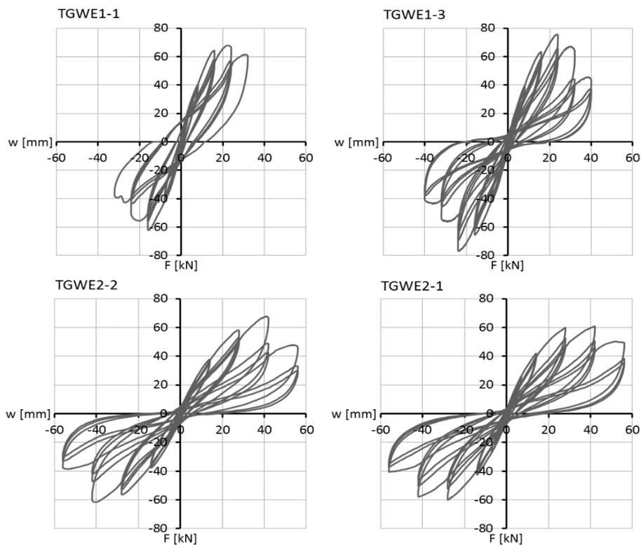
**Figure 11: F-w Diagrams for the Cyclic Horizontal Point Loaded Test Samples; a.) TGWE-1 (glass pane in one piece), c.) TGWE-2 (glass pane in two pieces),** Source: Ber et al. (2014)
