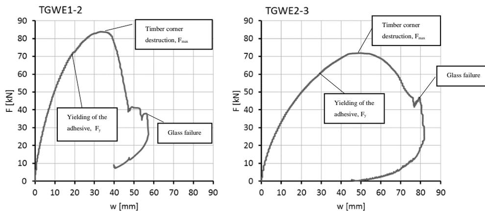
**Figure 10: F-w Diagrams for the TGWE-1 and TGWE-2 Test Samples Under Monotonic Horizontal Point Load, Source: Ber et al. (2014)**
