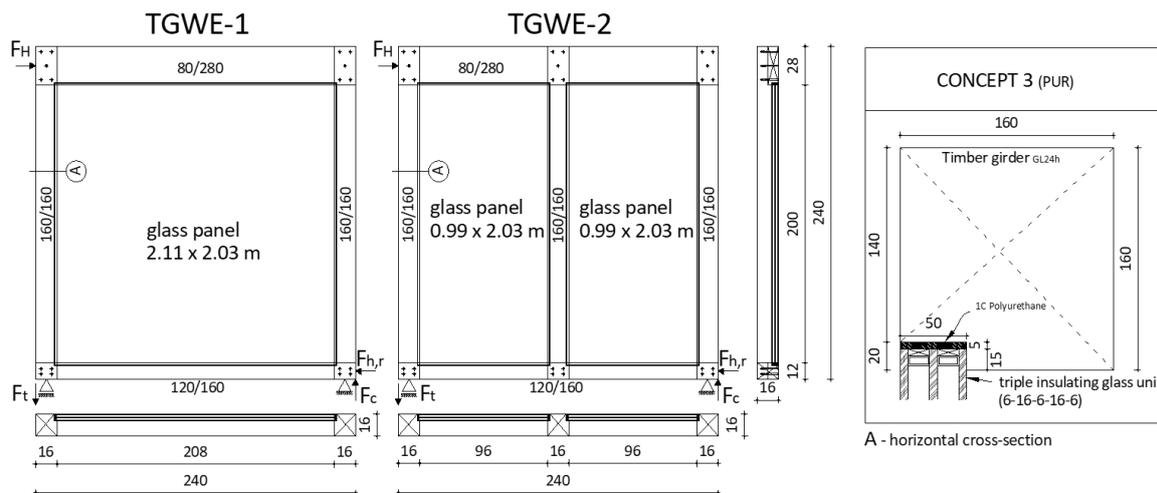
**Figure 8: Geometry of Both Testing Groups, TGWE-1 and TGWE-2, Source: Ber (2014)**
