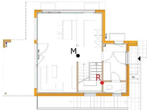
**Figure 2: Ground Floor Plan with Indicated Mass Centre (M) And Centre of Rigidity (R) Placed Away From Each Other**
