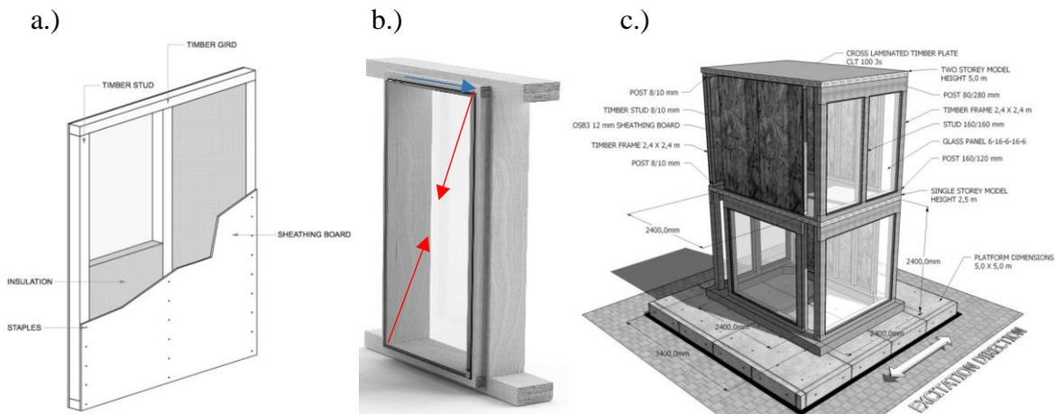
**Figure 4: A.) Timber Frame-Panel Wall Construction, B.) Timber-Glass Wall Construction, C.) 3-Dimensional Timber-Glass House Box Model**
