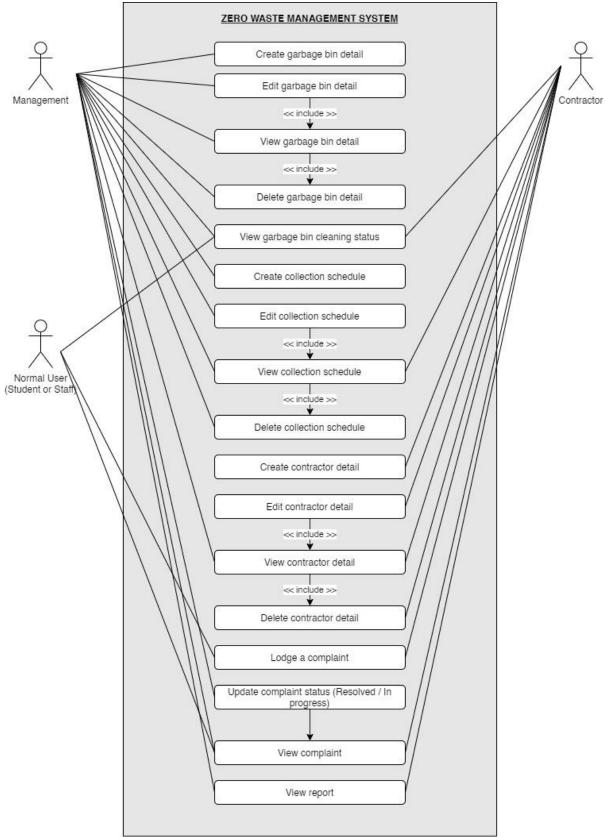
Figure 4: Use Case Diagram of the Proposed System
