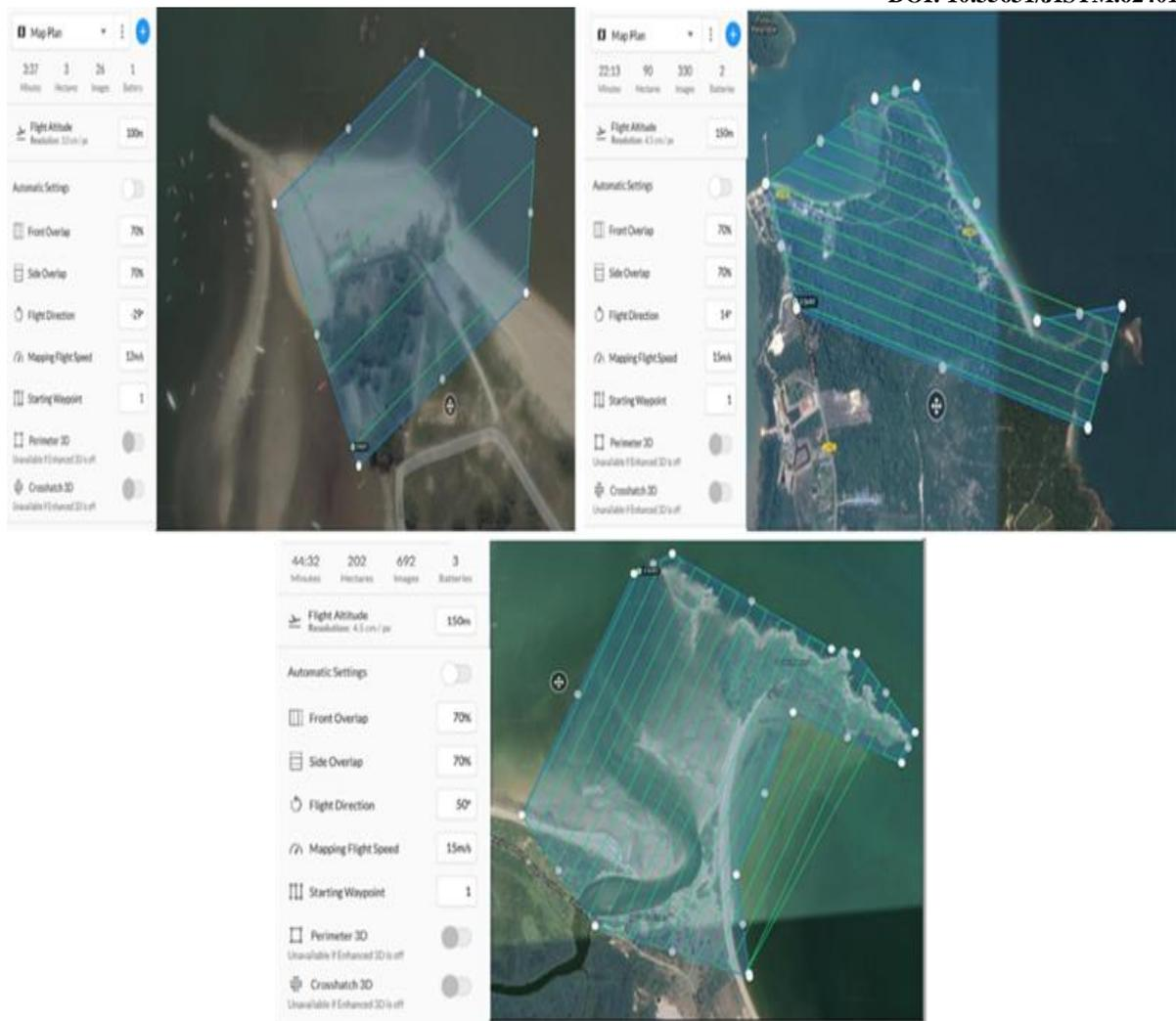
**Figure 6: Design of Flight Plan for This Study.**
