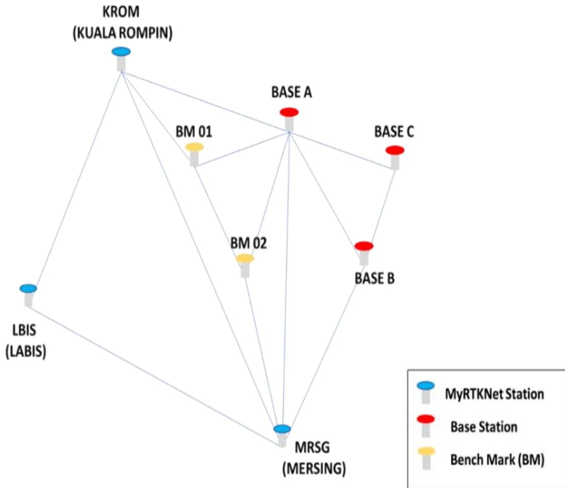
Figure 3: Design of the GPS Network Observation.
