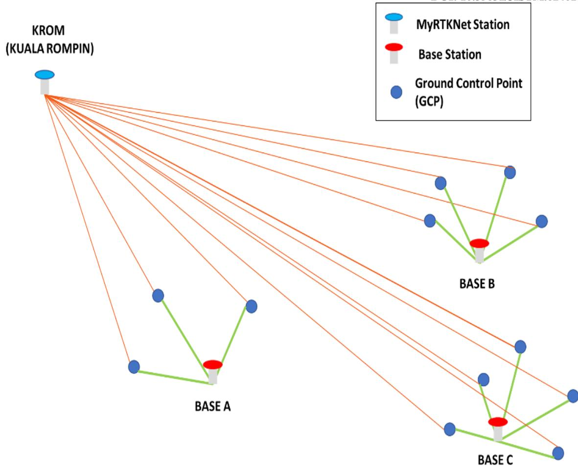
**Figure 4: Each GCP is Connected to the BASE and Checked Using KROM Station for Quality Assurance.**
