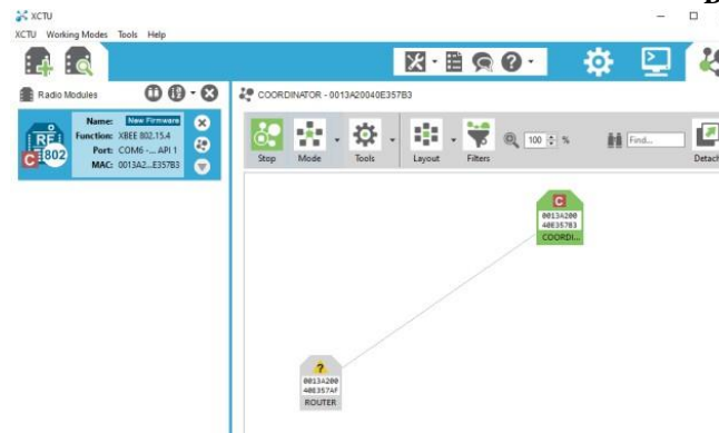
Figure 7: XCTU Software That Can Detect Other XBEE Devices In The Surrounding Area.
