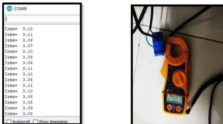
Figure 5: SCT 013 and AC Clamp Meter Value Measurement
