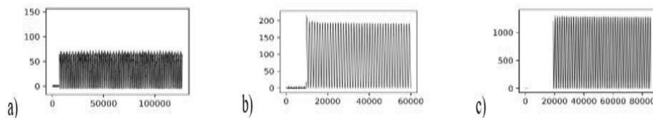
**Figure 7: Power Consumption Plots for (a) “Fan”, (b) “Hairdryer”, (c) “Heater”**
