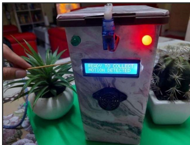
Figure 9: LCD Display Showing the Status “Ready to Collect” And “Motion Detected,” Where the Dustbin Lid Is Automatically Locked Real-Time Monitoring Using ThingSpeak
