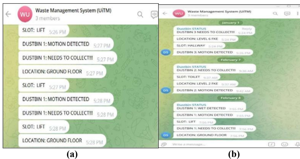
Figure 13 (A) And (B): Telegram Notification Alert Generated When The Bin Reaches The Threshold Level, Providing Real-Time Alerts for Waste Management Personnel
