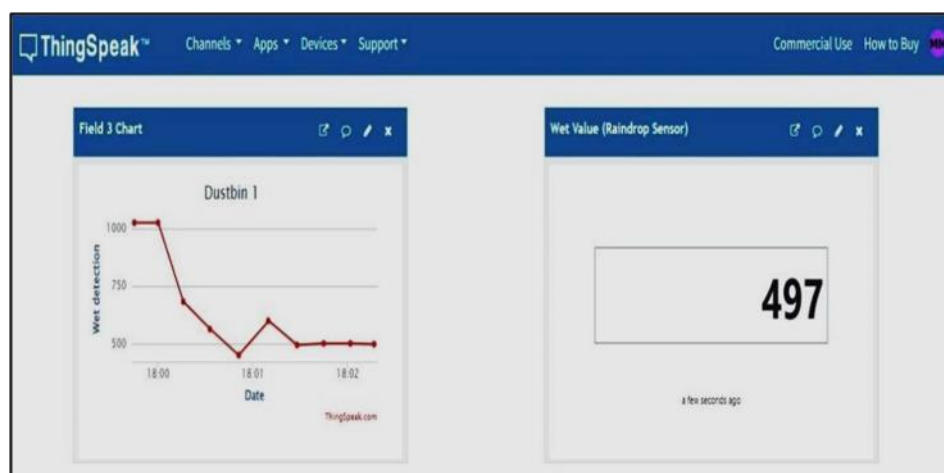
Figure 12: Real-Time Monitoring Graph on The Thingspeak Platform Indicating the Wetness Condition Within the Dustbin Based on Water Droplet Level Measurements
