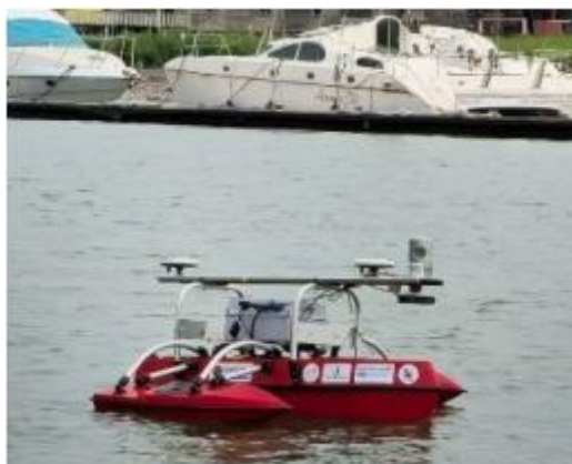
Figure 1: Sensors Deployed for Unmanned Surface Vessel (USV) Autonomous Navigation
