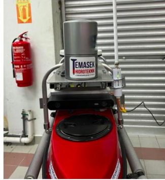
Figure 1: Velodyne LiDAR and ZED camera mounted on the survey vessel used for data acquisition in Klang, Malaysia.
