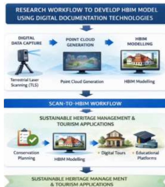
Figure 2: Research Workflow Illustrating the Integration of Digital Documentation Technologies For The Development Of An HBIM Model And Sustainable Heritage Management Applications.
