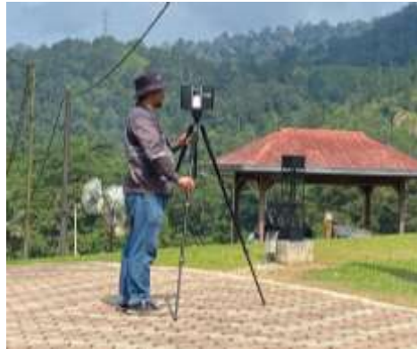
Figure 6: Terrestrial Laser Scanning Activities Using the FARO Focus M70 During Field Data Acquisition At Muzium Sungai Lembing
