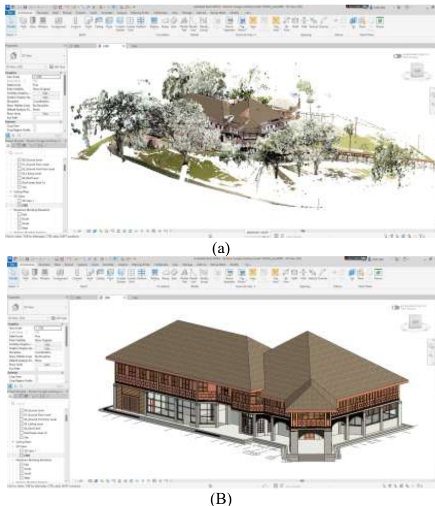
Figure 12: Three-Dimensional Visualisation of The HBIM Model Developed in Autodesk Revit: (A) Interior View With TLS Point Cloud Displayed For Geometric Reference, And (B) Completed HBIM Model With The Point Cloud Hidden
