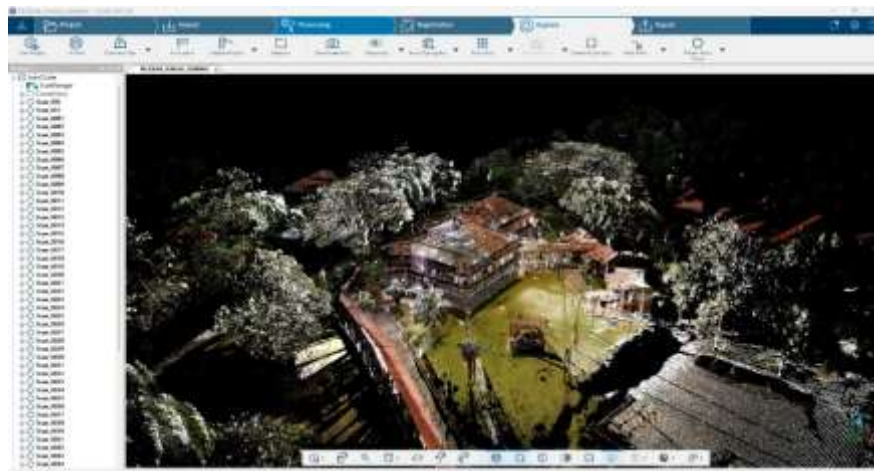
Figure 9: Registered TLS Point Cloud Dataset Of Muzium Sungai Lembing Generated Through FARO SCENE, Illustrating The Complete Three-Dimensional Spatial Representation Of The Heritage Building
